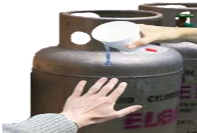
Figure 3.3 How the gas level is checked [3]
